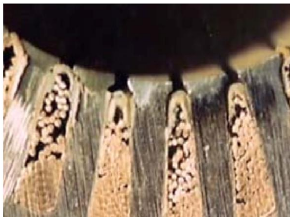
Figure 12. Low and improper stator winding slot fill
